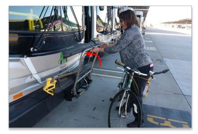
If the rack is empty, squeeze the handle and close the rack in its upright position.
