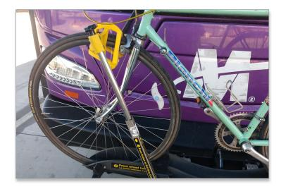
Release the arm so it secures the wheel to the rack.
