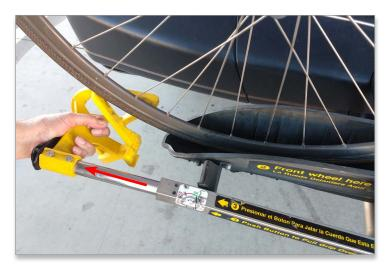
An extendable "arm" helps secure the front wheel of the bike.
